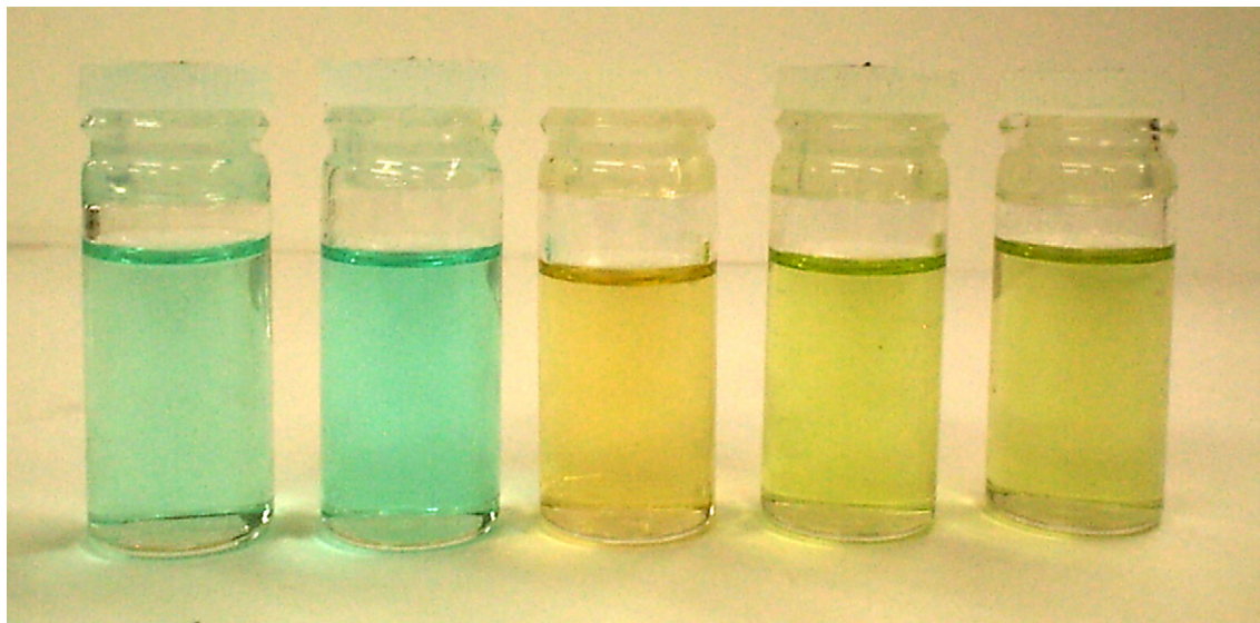
Fig. 4. The colors of \text{CH}_2\text{Cl}_2 solutions containing \text{H}_2\text{tppc} , [\text{Cu}(\text{tppc})] , [\text{Sb}(\text{tppc})\text{Cl}_2]\text{SbCl}_4 , [\text{Sb}(\text{tppc})(\text{OH})_2]\text{PF}_6 , and [\text{Sb}(\text{tObpc})(\text{OH})_2]\text{PF}_6 (on going from the leftmost to the rightmost). (For interpretation of the references to color in this figure legend, the reader is referred to the web version of this article).
